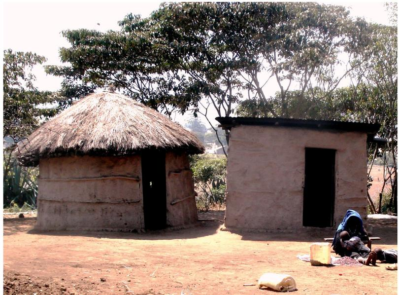
Figure 2: Typical Wattle and Daub construction at a compound in Musa. Here also illustrates an example of both a thatch roof (left) and corrugated metal roof (right) (Reineccius 2012).
